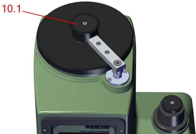
Figure 10: Showing top of Gasometric Drum (10) with Calibration Weight receptacle (10.1)
