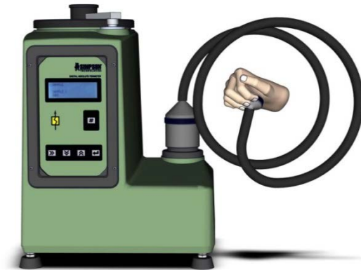
Figure 5.5.1 – Showing sealing of the Mold Permeability Accessory with hand
