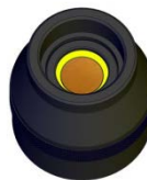
Specimen Retaining Ring with Sand and Spacer inserted into accessory
