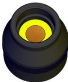
Specimen Retaining Ring with Sand Specimen inserted into accessory
