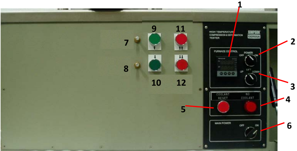
Figure No. 2 Tester Front Panel
