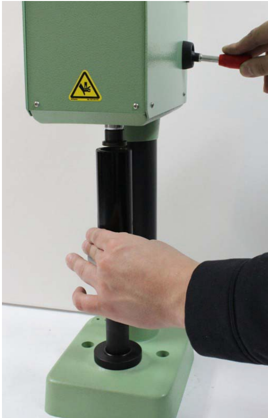
Figure 7: Preparing a Sand Specimen
