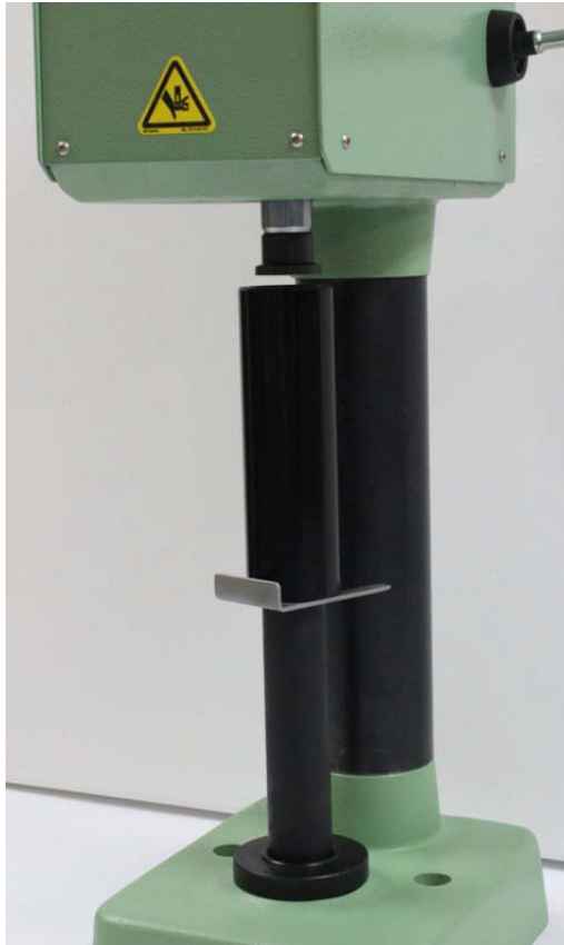
Figure 6: Specimen Tube Assembly in Rammer Ready for Testing
