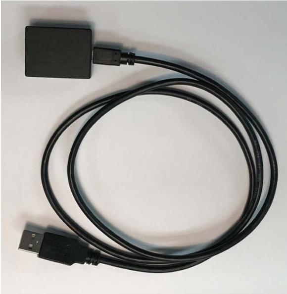
**Figure 3: USB Cable and Infrared IR Receiver**
