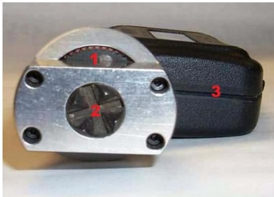
**Figure 6: Collar (1) Penetrator (2) and Body (3)**
