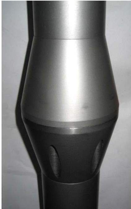
Figure 2: Showing the coupling hubs of the two sections of the shatter index tester.
