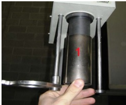
Figure 10: 2" x 2" (50 mm x 50 mm) specimen tube (1) positioned on the Shatter Index Tester stripping post
