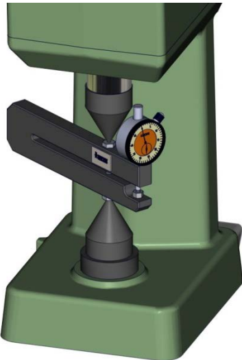
Figure 9: Mechanical load cell slightly compressed between the upper and lower supports
