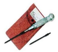
For the determination of the safe curing time for molds and cores made of cold-hardening sand mixtures.
