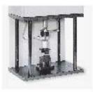
Twin Transverse Shear Strength on standard specimen Ø 50 x 50 mm or Ø 50,2 mm x 2 inches
